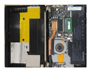
2. Disassemble the battery strip and uesd a screwdriver remove the battery screws, heat dissipation module, fan, SSD, motherboard, and small board screws.
